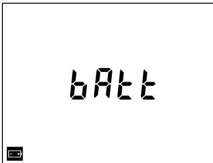
Figure 5: The low battery indicator signals the need for a replacement.
