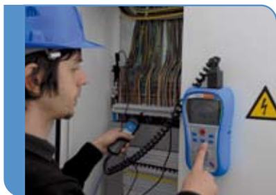
Magnetic holder for hands free operation
